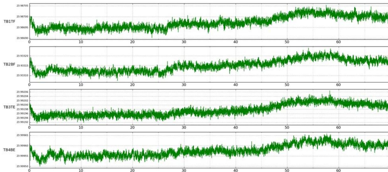
Figure 10 - Close up of data strip showing test mass control within a 0.15 milli-K band for 70 hours. Ambient temperature varied approximately +/- 1°C during this run. X-axis is hours, Y is °C.
