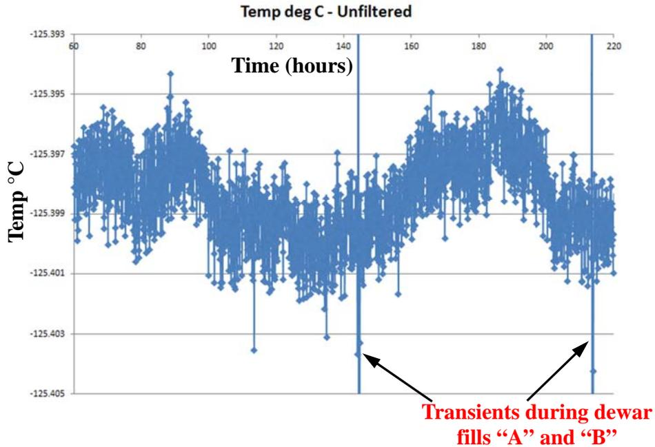
Figure 15 – CCD Simulator Temp – Unfiltered data from Isotech 125
