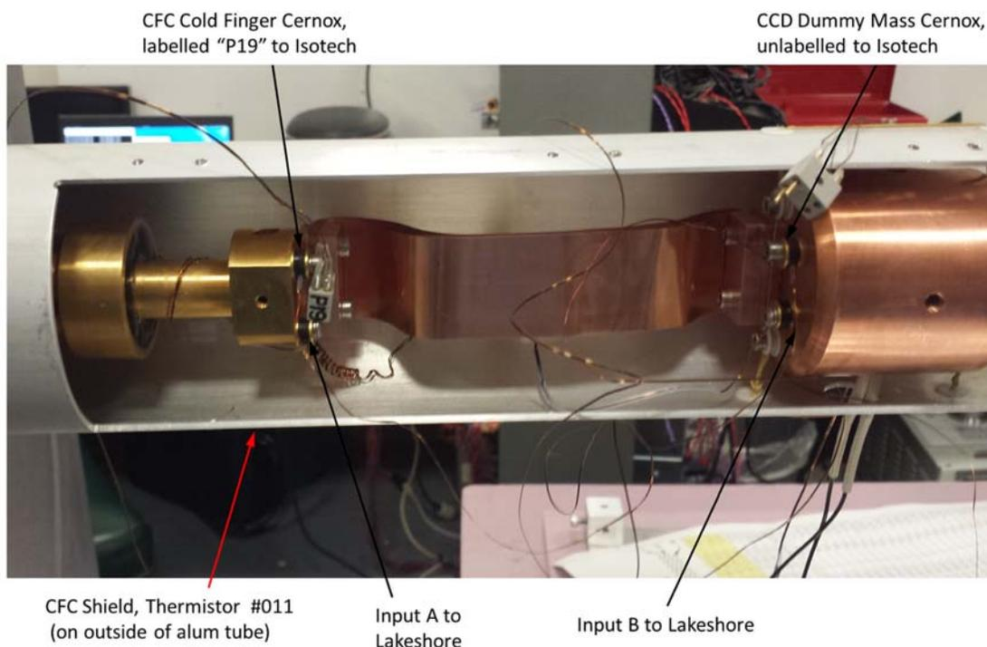
Figure 11 – CFC Cold Finger and CCD Dummy Mass Test Set-Up
