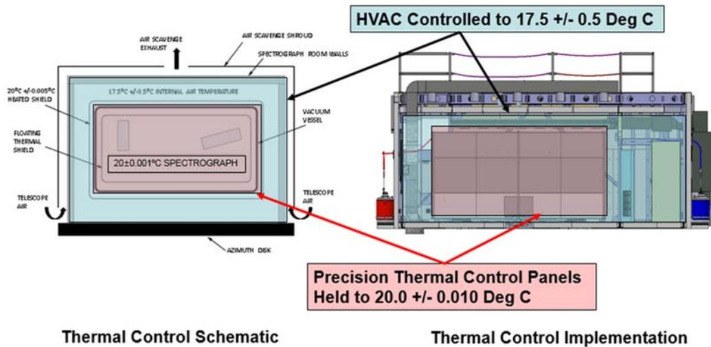
Figure 1 – Spectrograph Thermal Control Strategy
