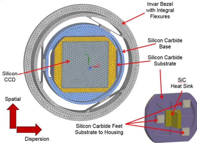
Figure 6 – Thermal/Structural Model of the Focal Plane
