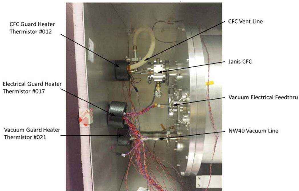
Figure 12 – Penetrations and Guard Heaters
