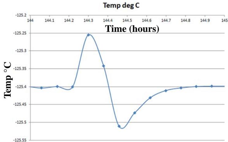
Figure 16 – CCD Simulator after fill event “A” – Temperature recovery in ~1/2 hour
