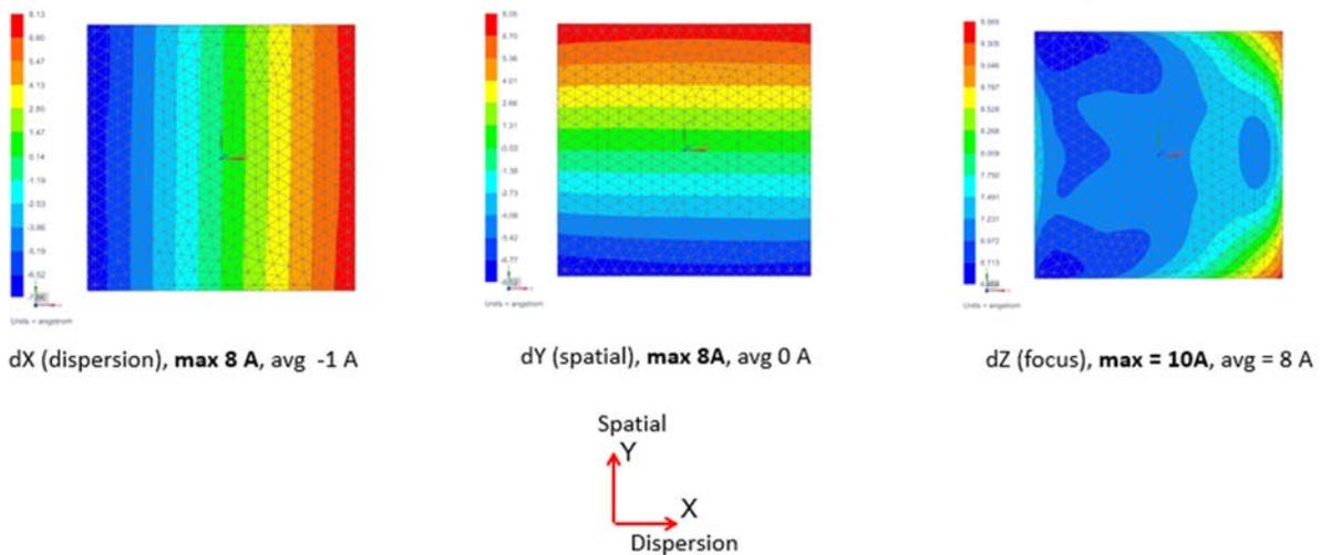
Figure 7 – CCD Displacement Results from Structural Model Using Temperature Mapping from Thermal Analysis
