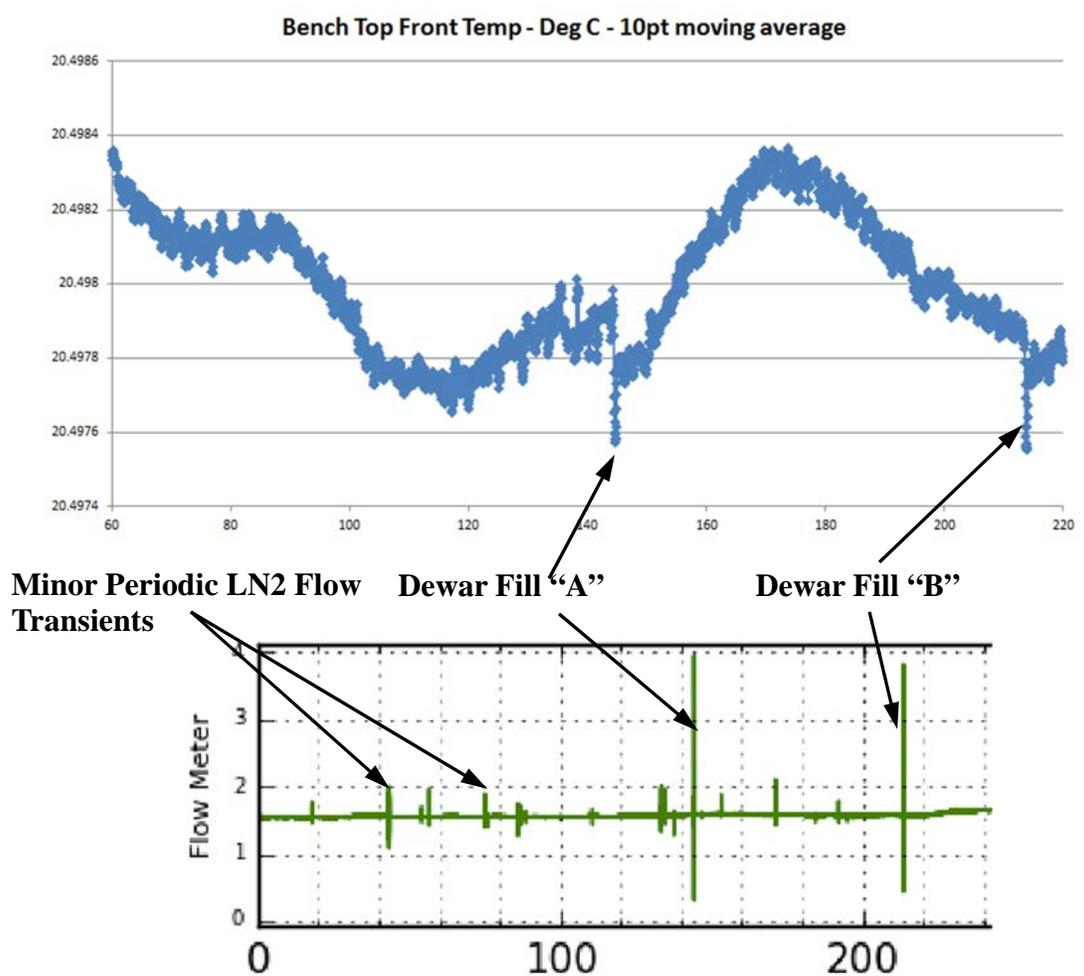
**Figure 14 – Bench held within a .001 K band for 160 hours (6.7 days). X-axis for both panels is “hours”, Y is “°C” for upper panel and “lpm gas” for lower panel. Ambient varied by ~2°C (18.5°C to 20.5°C).**
