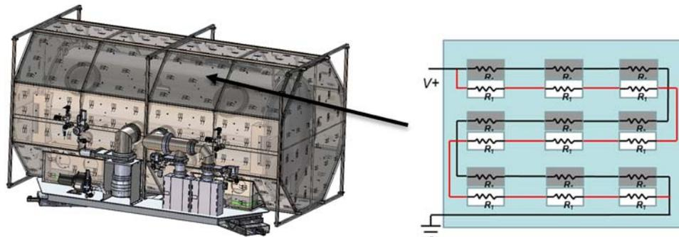
Figure 2 – Thermal Panel Assembly (Left) with a Schematic of a Typical Heater Panel (Right)
