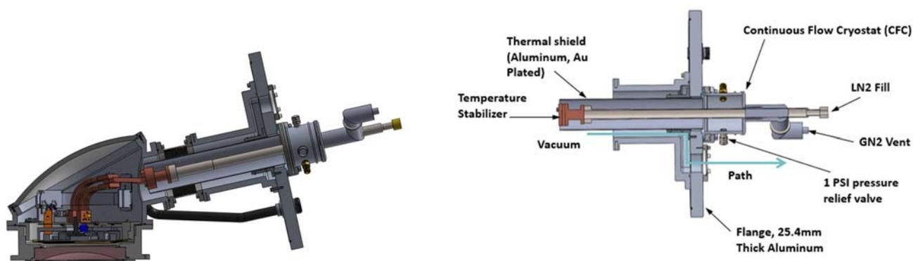
Figure 4 – Continuous Flow Cryostat (CFC) Connected to Focal Plane
