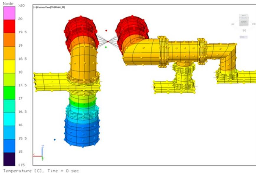
**Figure 8 – Thermal Modeling of Vacuum Feedthroughs**
