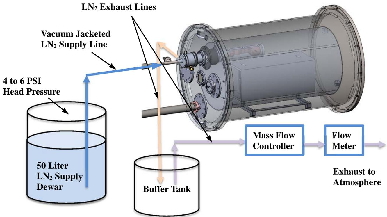
Figure 13 – LN<sub>2</sub> Flow Control Schematic
