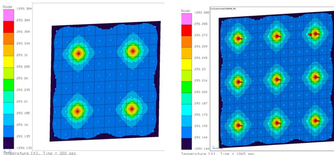
Figure 5 – 4 and 9 Heater Panel Analytical Models
