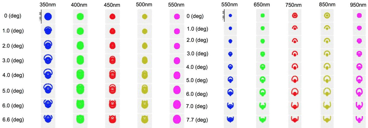
Figure 14: Camera performance outside of the Spectrograph mainframe. Left/Right: Blue/Red Camera; Box size=100µm.
